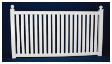
Rails: 2" x 3-1/2" Top & Bottom Rail (Reinforced) 2" x 3-1/2" Mid Rail (on 6' ht. only) Pickets: 7/8" x 3" Pickets Picket Space = 1-5/8"
