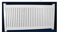
**Rails:** 1-1/2" x 5-1/2"Top & Bottom Rail (Reinf) 2" x 3-1/2" Mid Rail (on 6' ht. only) **Pickets:** 7/8" x 3" Pickets Picket Space = 1/2"
